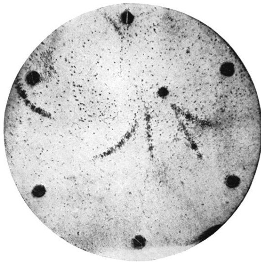
FIG. 3. A group of six particles projected from a region in the wall of the chamber. The track at the left of the central group of four tracks is a negatron of about 18 million volts energy ( H\rho = 6.2 \times 10^4 gauss-cm) and that at the right a positron of about 20 million volts energy ( H\rho = 7.0 \times 10^4 gauss-cm). Identification of the two tracks in the center is not possible. A negatron of about 15 million volts is shown at the left. This group represents early tracks which were broadened by the diffusion of the ions. The uniformity of this broadening for all the tracks shows that the particles entered the chamber at the same time.
